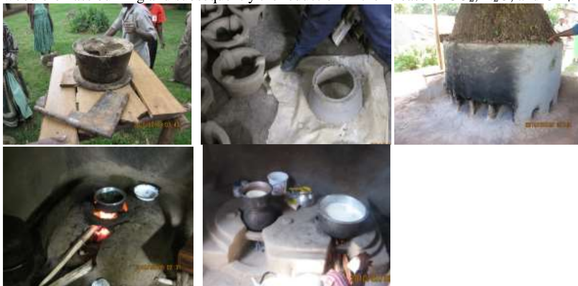
Figure 3. The metal mold (upper left), finished soft ceramic liners (upper middle), kiln (upper right), installed one-pot stove (below left), and two-pot stove (below right)
