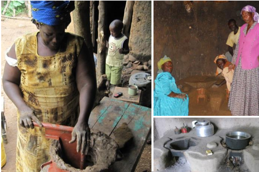
The Upesi cook stove, produced and installed locally by women, replaces the 3-stone.
